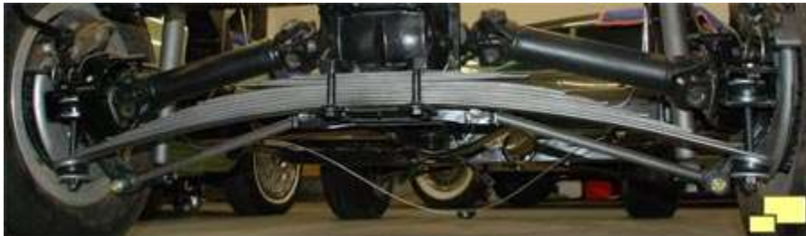
Steel multi-leaf transverse spring in rear of a C2 Corvette.
