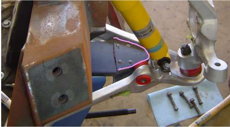
C4 front suspension from a restomod project, minus the swaybar and with one end of spring sitting on the A-arm pad highlighted with pink for clarity.
